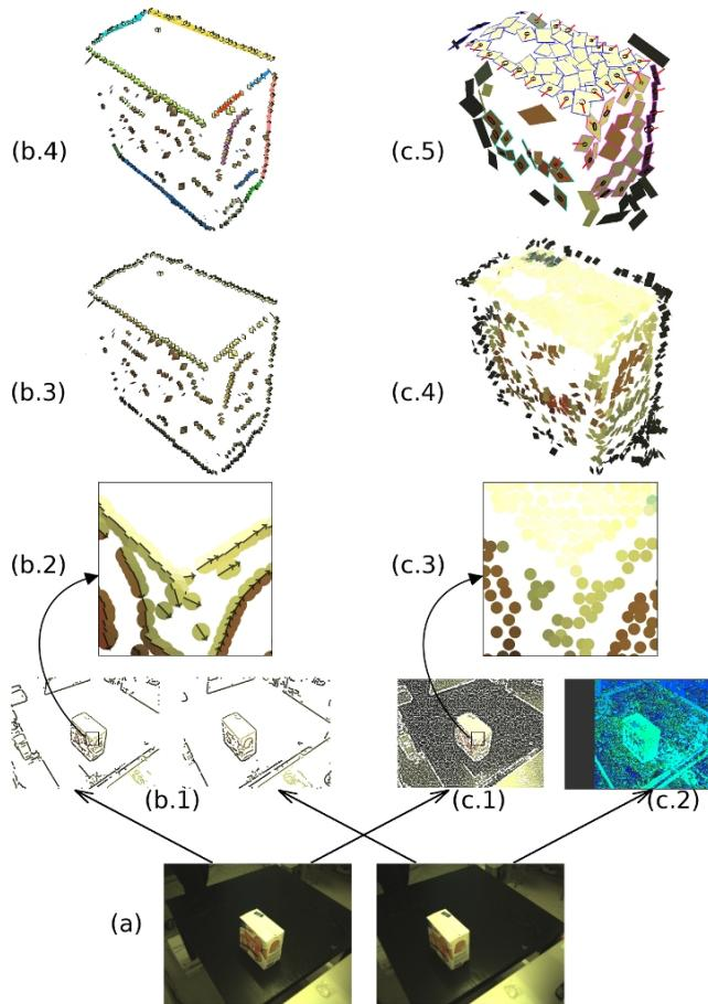
Fig. 2: The hierarchical representation of edge and texture information in the ECV system. (a) An example stereo image pair. (b.1) 2D line segments for the left and the right image. (b.2) a detail from b.1. (b.3) 3D line segments. (b.4) 3D contours. (c.1) 2D texlets for the left image. (c.2) disparity image. (c.3) a detail from c.1. (c.4) 3D texlets. (c.5) 3D surfings segmented into three surfaces, see also figure 4. This figure is best viewed in color.
