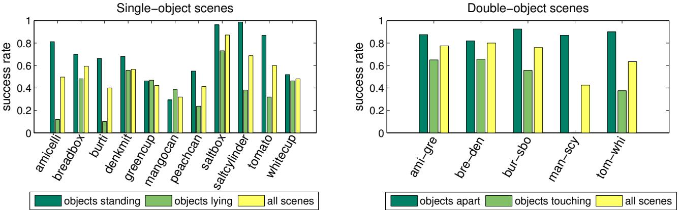
Fig. 8: The combined-grasp success rates per object. One grasp of each of the six grasp type is attempted. For the single-object scenes, the results are shown for the objects standing up and lying down, whereas for the double-object scenes, the results are given for the scenes with the objects apart and touching.
