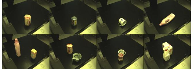
Fig. 5: Experimental scenes, left camera images. Top row: single object scenes. In the first two images (from left to right) objects are in upright position, in the last two images objects are laying down. Bottom row: scenes with two objects. In the first two images objects are placed apart from each other, in the last two images they are close by.
