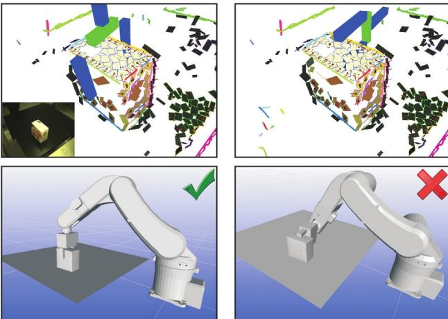
Fig. 3: Examples of two different grasps. The grasps are generated based on the ECV representation of the real scene (first row). The grasps are then tested in a simulated environment (second row). The grasp in the first column results in a successful grasp, whereas the grasp in the second column fails.
