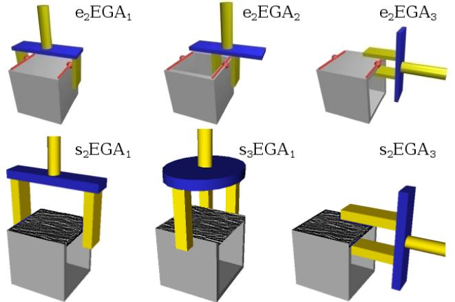
Fig. 1: The elementary grasping (EGA) actions. Top row: three types of edge-based EGAs. The red lines indicate the selected contours. Bottom row: three types of surface-based EGAs. The dark face shows the selected surface.
